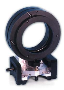
OMS 160 is an optical mount for non-standard optical lens with outer diameter of 160 mm featuring similar mechanical design as OMS 120. It has a 4-axis movement capability: 2 linear displacements (x, y directions) and 2 independent angular positioning. The system can be mounted on a standard optical rail or table. The mount is fabricated from aluminium and murytal.
