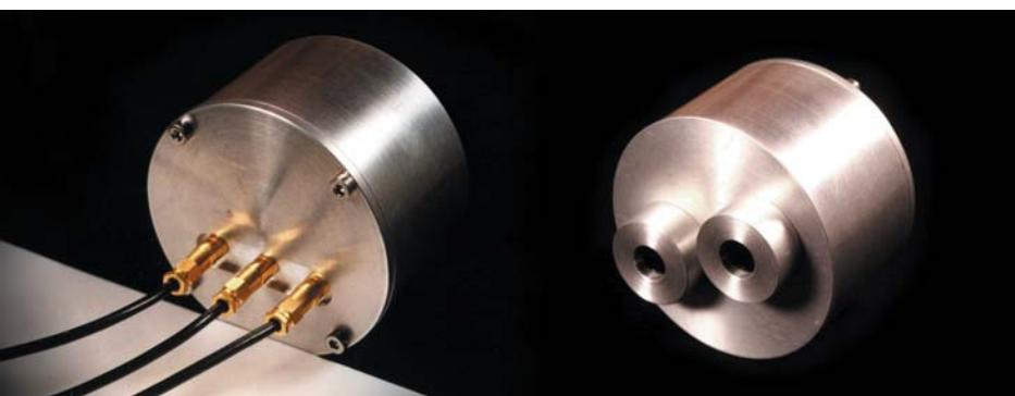
The DP 1310 fast IR detector was developed for measurement and monitoring of the laser double-pulse delay. The mechanic design allows simple implementation of various spectral filters.
